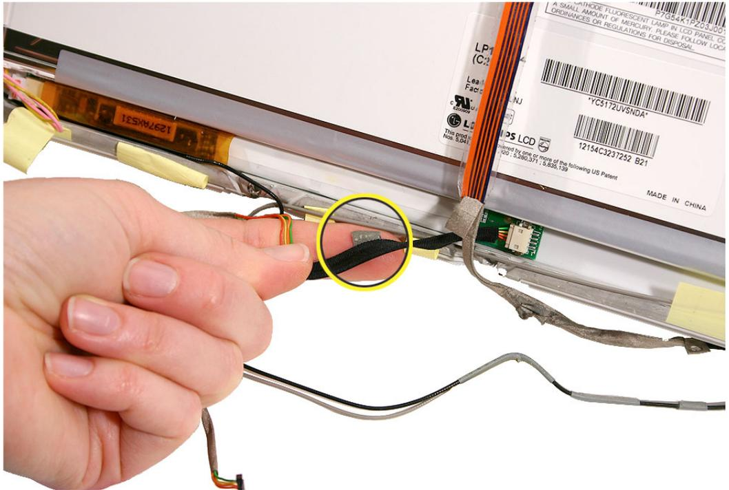
8. Note how the gray cable is routed along the bottom of the inverter board, under the bezel brace, and around the corner by the corner tab.
