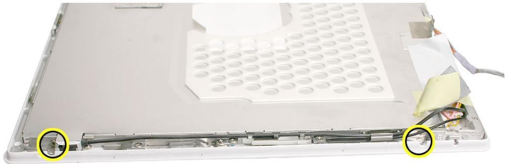
5. Peel up the tape that holds the shield to the bezel brace.
