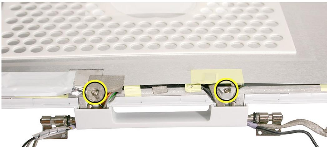
**Important:** Note that one of the screws (left side of the clutch when the display is oriented as shown) also has a washer. Be sure to reinstall it before installing the clutch cover screw.
