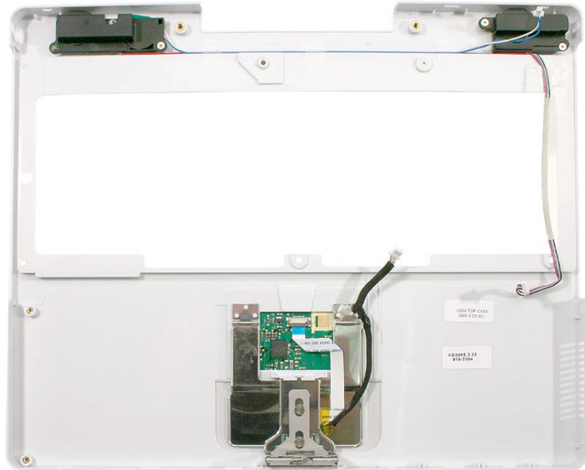
**Important:** Make sure you transfer the original serial number label and Ethernet label from the old top case to the replacement top case. You can use a black stick to carefully peel up a corner of the label. Then peel off the label completely and apply it to the replacement top case. Make sure that the labels lie completely flat so they do not interfere with the battery compartment.
