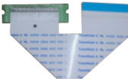
3. If the cable has another supplier's designation, disconnect the cable from the logic board and check the underside of the cable for yellow tape that covers the cable in the area shown.
