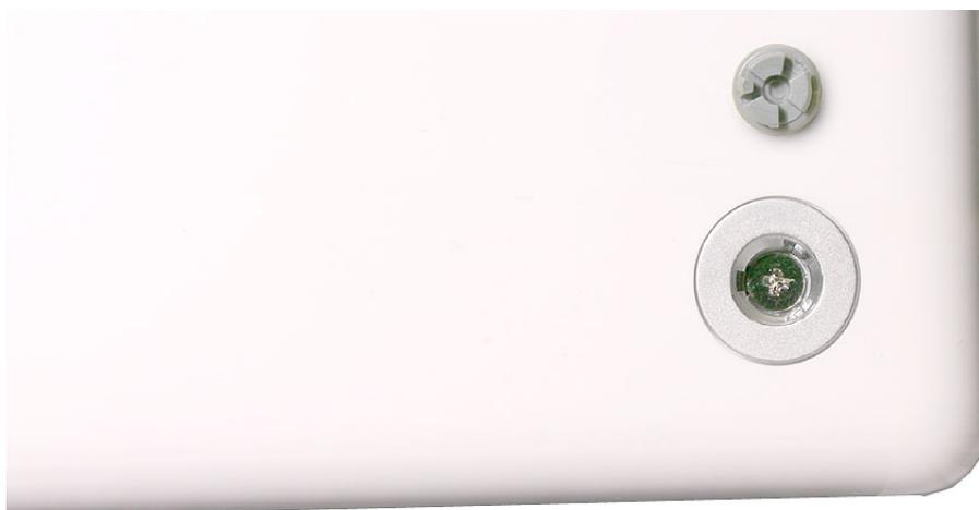
5. **Important:** To avoid damaging the case, be careful that the screwdriver tip does not slip out of the screw head during removal.
