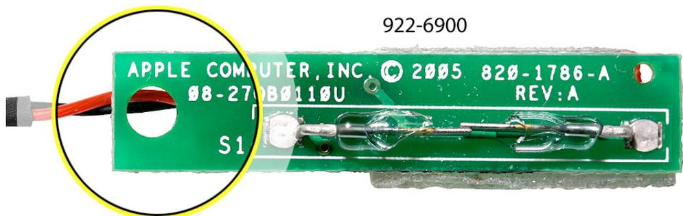
2. If the cable is soldered to the front side of the board and the spacer has been eliminated (as shown below), it is the newer version (922-7829) and no replacement is required.
