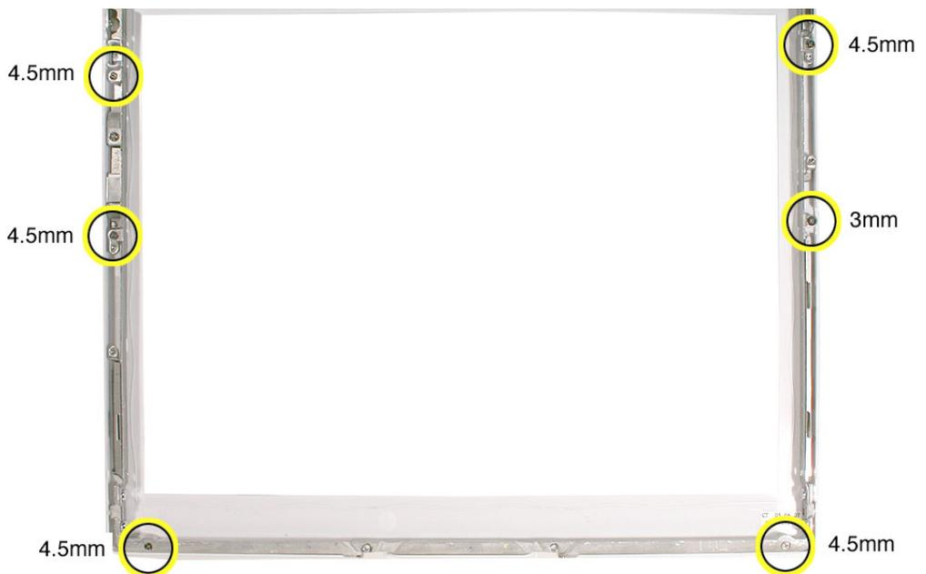
**Replacement Note:** Install screws in a counter-clockwise direction, starting at the top left corner of the bezel brace.
