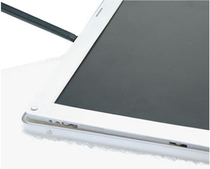
3. Lift off the display assembly from the display housing.
