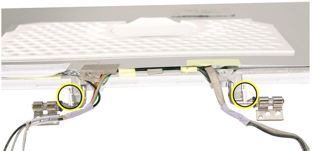
4. Note the proper placement of the left and right clutch caps. The caps are unique for each side and are not interchangeable. A molded marking on the inner side of the clutch caps helps identify their intended location in the display assembly. For instance,
