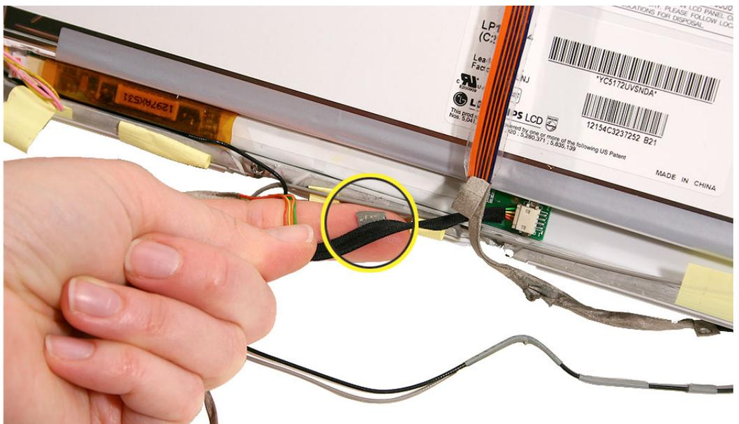
4. Use a black stick or flat-blade jeweler's screwdriver to disconnect the inverter cable from the inverter board.
