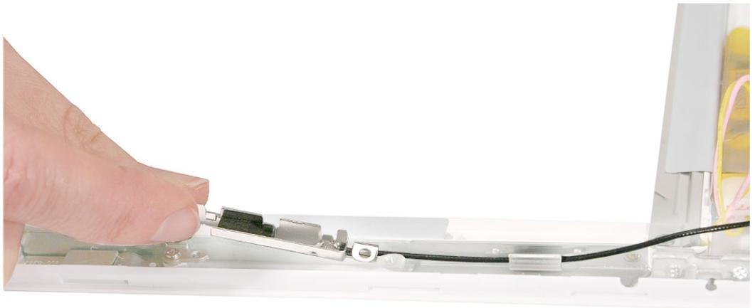
7. From the bottom of the bezel, lift up the inverter cable where the mesh tab anchors the gray antenna cable between the bezel brace and the inverter board.
