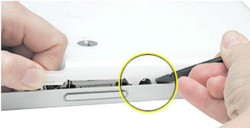
10. Carefully work the black stick around the corners of the bottom case.
