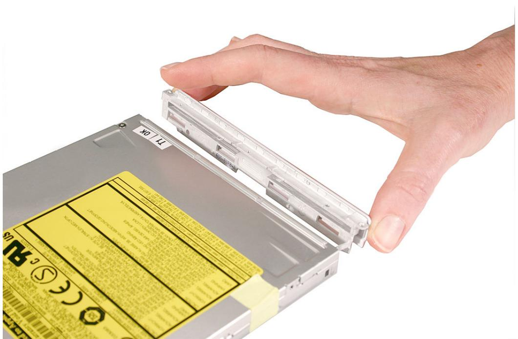
12. Install the replacement optical drive, and reassemble and test the computer.
