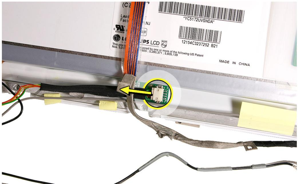
5. Install the replacement inverter cable and tape, and reassemble and test the computer.
