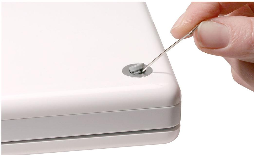
3. Remove the three identical Phillips screws from the metal sockets.
