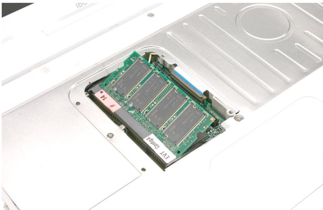
4. Align the notch in the replacement memory card with the small tab in the memory slot. Hold the card at a 30-degree angle, then push the card into the slot until it is firmly seated.
