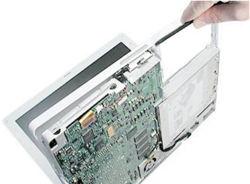
8. While continuing to loosen the top case, use caution around the battery bay. If necessary, flex the inner frame to release that corner of the top case.
