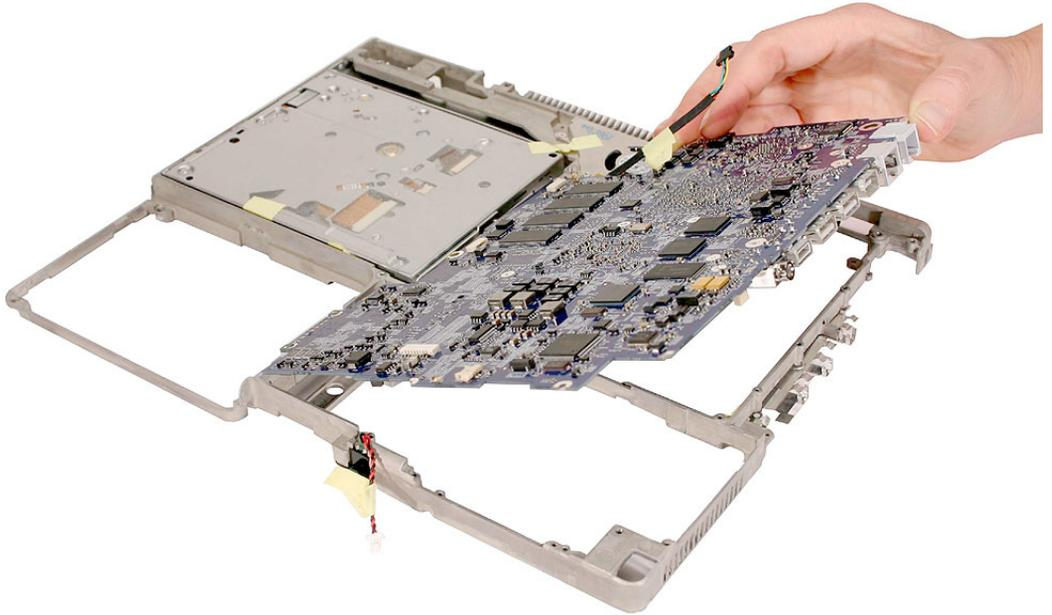
6. Install the replacement logic board, and reassemble and test the computer.
