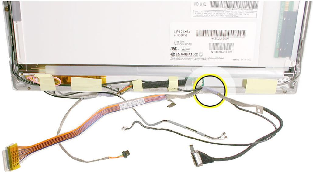
4. Remove the LVDS cable from the bezel assembly.
