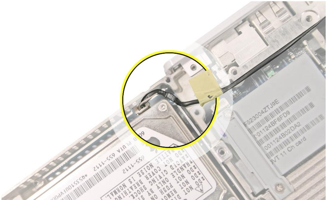
5. Press in on the upper bracket to clear it from the frame. While pressing on the bracket, use a black stick to begin to lift up the end of the hard drive.
