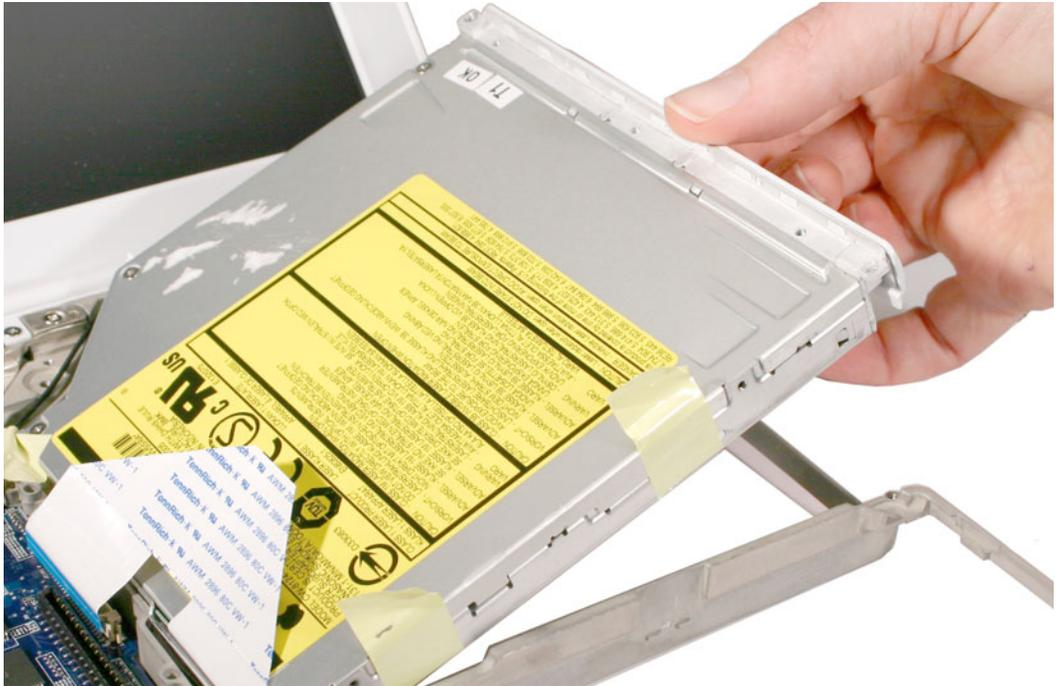
6. When removing the drive, the bottom of the drive case might stick to tape on the underside of the frame. If it does, use a black stick to release the drive.
