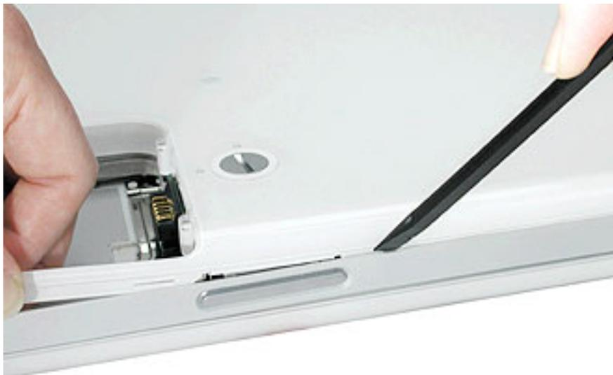
9. **Warning:** To avoid damaging the sleep light and other delicate components, do not insert the black stick too far into the computer as you free the bottom case from the computer. Use just the tip of the black stick to pry up the bottom case.
