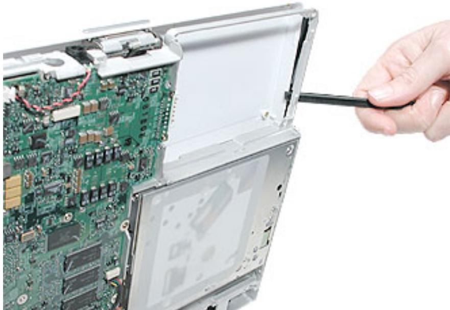
9. **Warning:** The top case is connected to the computer assembly with delicate cables. Do not remove the top case until the cables are disconnected (see the next steps).
