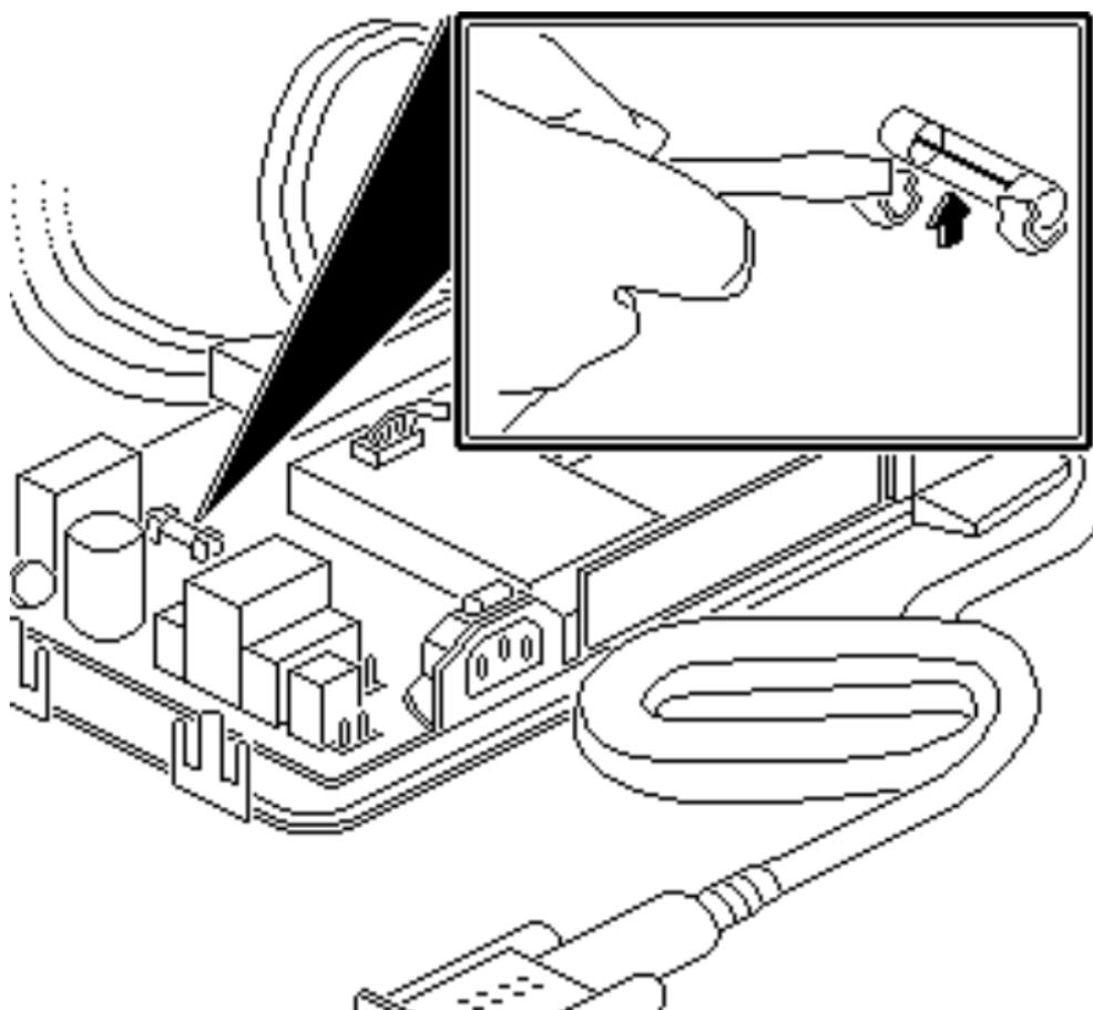
Using a small, long-stemmed screwdriver, pry up one end of the fuse and remove it from the main board.
