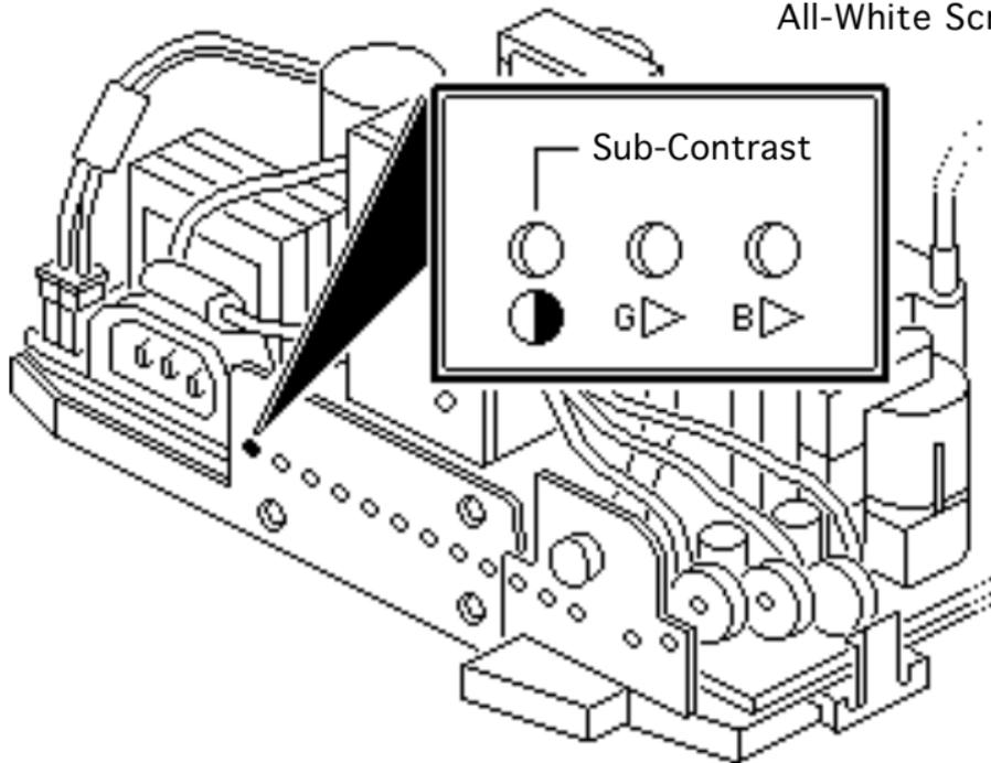
8 Using the light meter and a two-inch plastic screwdriver, adjust the sub-contrast control until you get 30 foot lamberts ( $\pm 3$  foot lamberts), which on the light meter is
