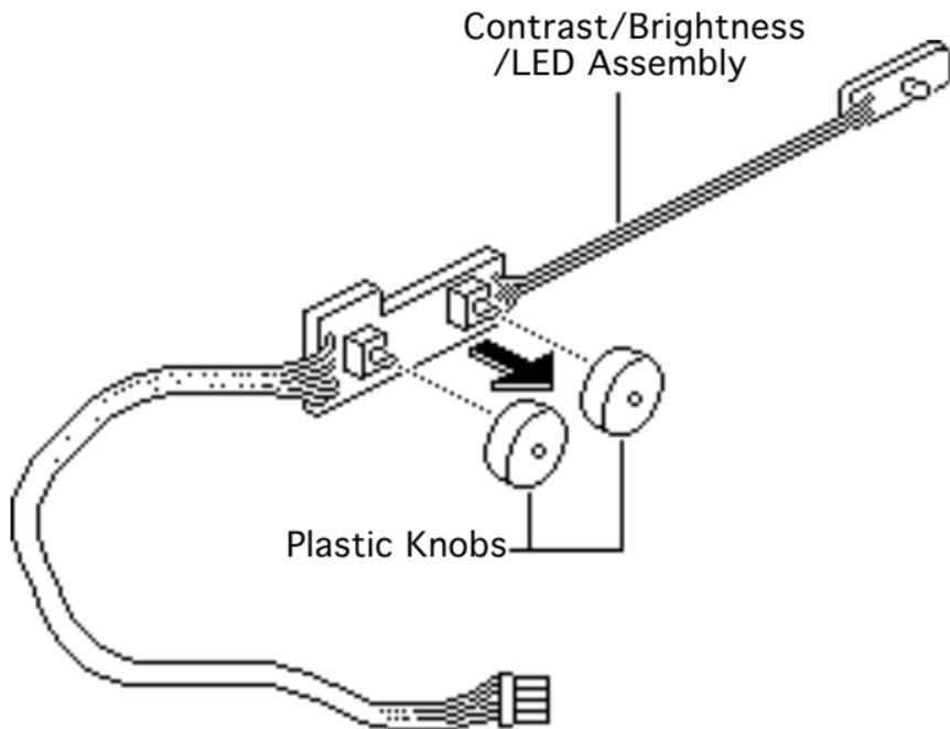
**Replacement Note:** If you are replacing the contrast/brightness/LED assembly, remove the plastic knobs and reinstall them on the new contrast/brightness/LED assembly.
