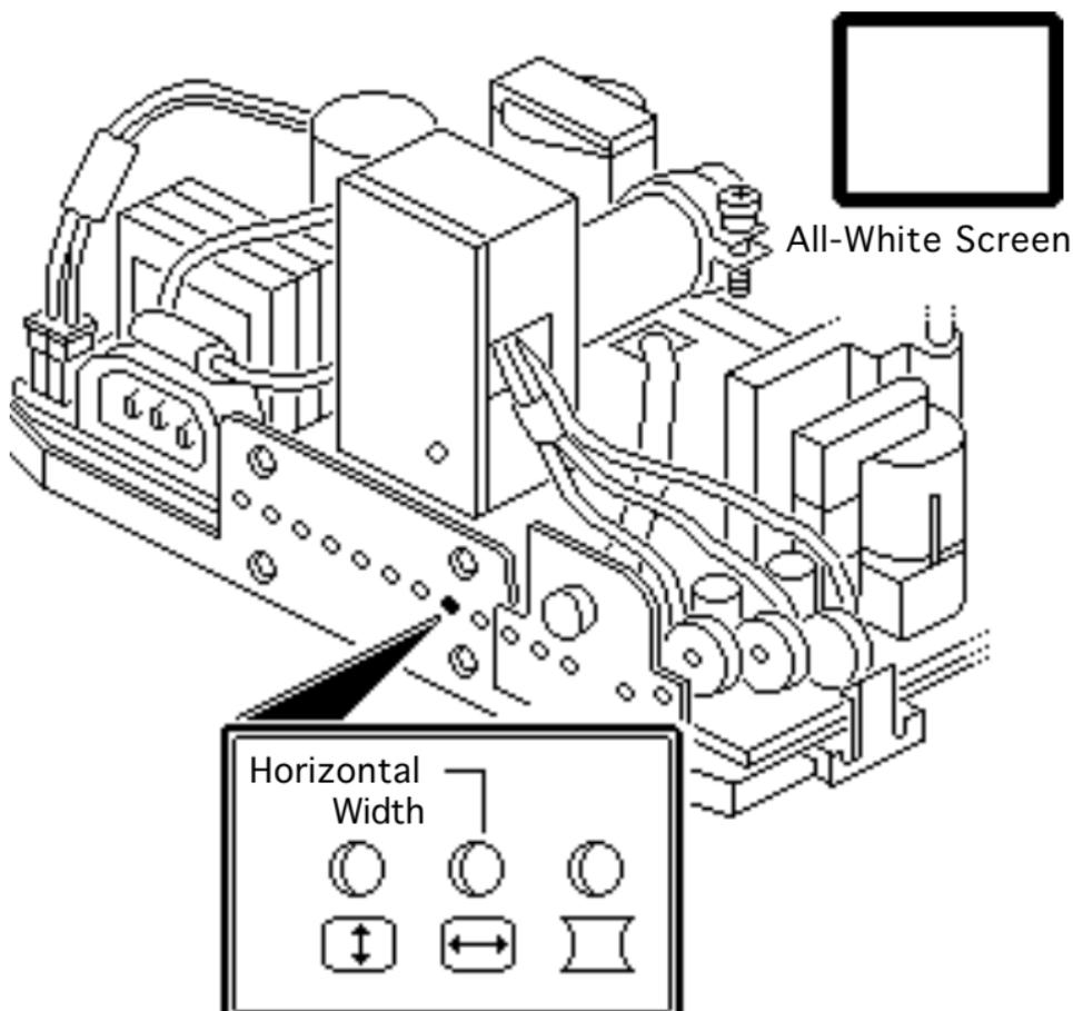
Using a hex-head plastic adjustment tool, adjust the horizontal width control until the raster is 9 1/4 in. ( $\pm 1/8$  in.) or 235 mm ( $\pm 2$  mm).
