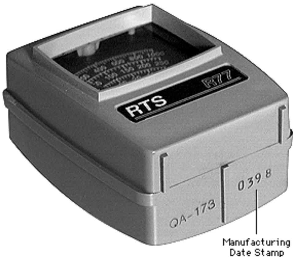
readings, verify the readings with a known-good light meter or photometer. Also check the age of the R77 light meter by its four-digit manufacturing date stamp (such as 0398 for March 1998).
