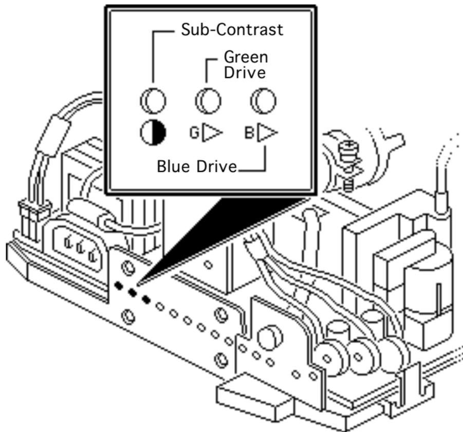
**Note:** To set the green and blue drive controls to their 3/4 position, turn the controls to their full clockwise position and then turn back 1/4 turn counterclockwise.
