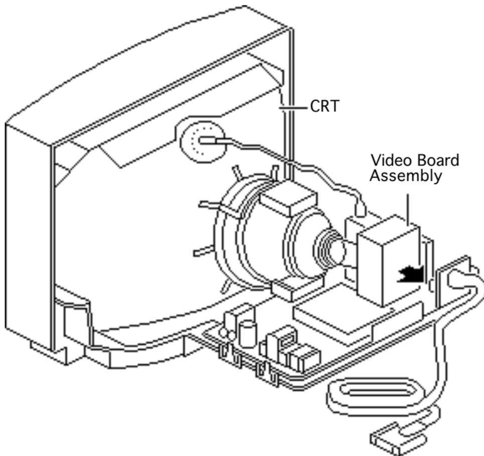
**Caution:** Twisting, bending, or applying force to the video board assembly could damage the neck of the CRT. Be sure to pull the CRT/video board straight off the CRT.
