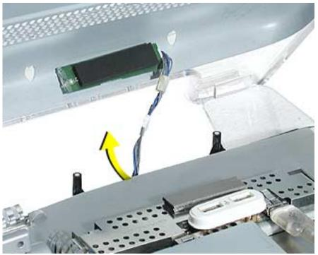
3. Carefully pull the ADC cable through the hole in the rear cover.
