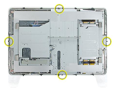
2. Carefully lift the display panel off the front bezel **Note:** The display panel is very heavy. Use caution when lifting the panel out of the bezel.
