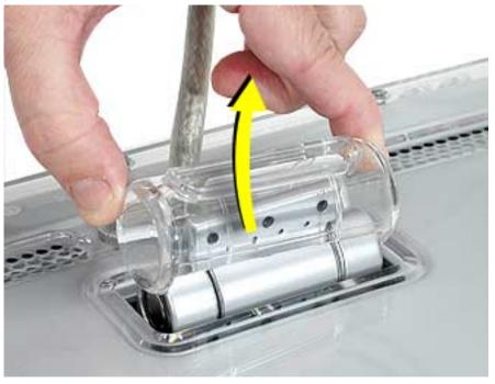
3. Pull the ADC (Apple Display Connector) cable through the opening in the foot to separate the foot and the cable.
