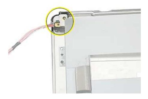
4. Carefully slide the top bulb tray out of the panel. **Note:** The top and bottom bulbs are interchangeable.
