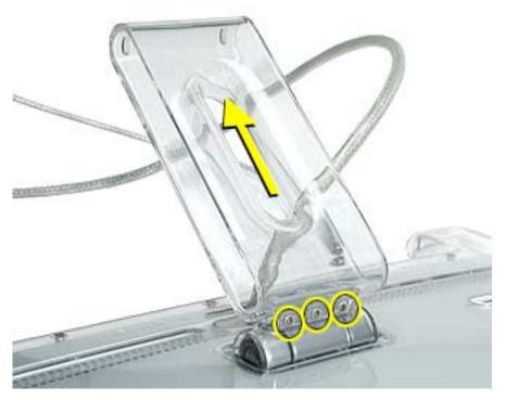
2. The clear hinge cap may fall off the foot. If it doesn't, remove the hinge cap from the foot.
