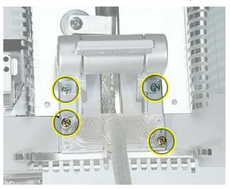
2. Pull the ADC cable out of the way and remove two more hinge screws.
