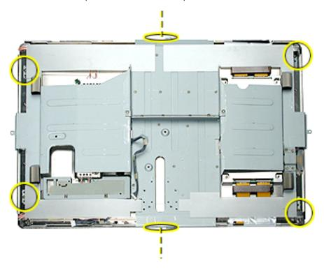
2. Pull the cable (circled below) through the hole in the chassis, then lift the metal chassis off the LCD panel.
