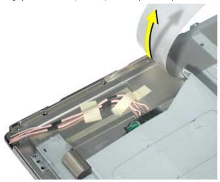
2. Release the masking tape and disconnect the two bulb cables from the inverter board.
