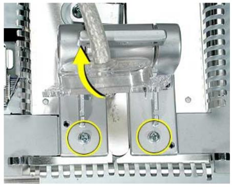
3. Lift the hinge up and off the chassis. **Replacement Note:** The hinge has locators on it, so it seats correctly in the chassis.
