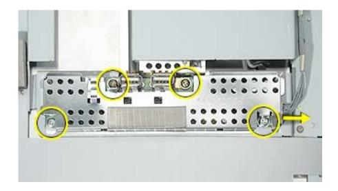
3. Lift the USB board (located inside the shielding) from the chassis. Remove the USB shield and copper ground shield. **Note:** The shielding needs to be removed before returning the USB board to Apple.
