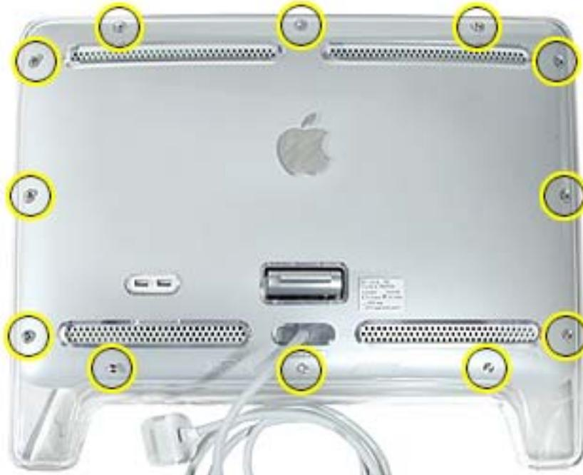
2. Lift the rear cover from the top to help disengage it from the tabs on the front legs.
