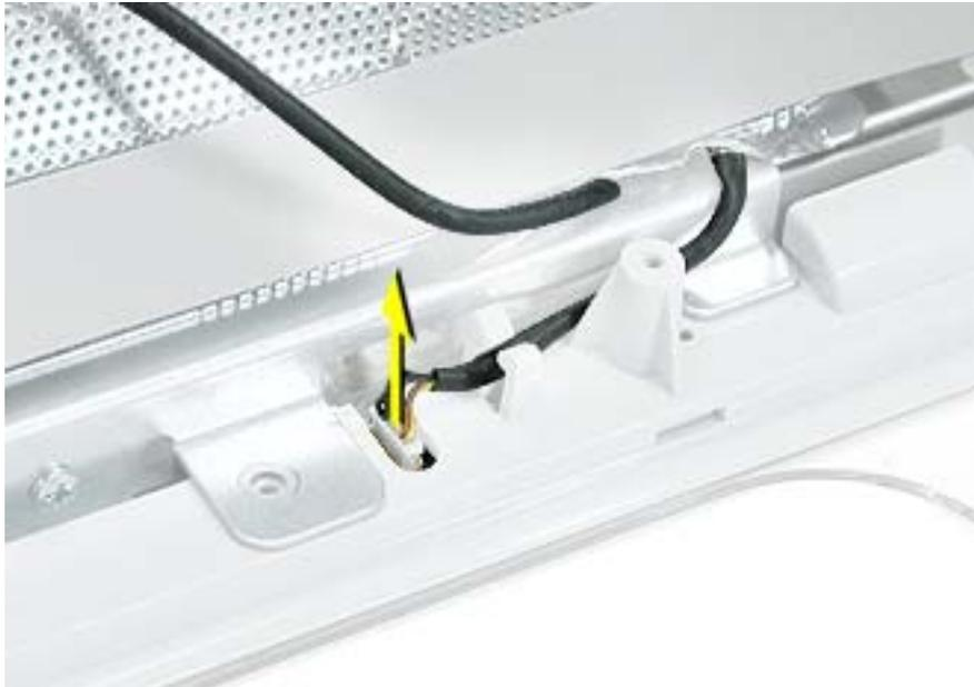
3. Carefully separate the wire clips enough to remove the wires.
