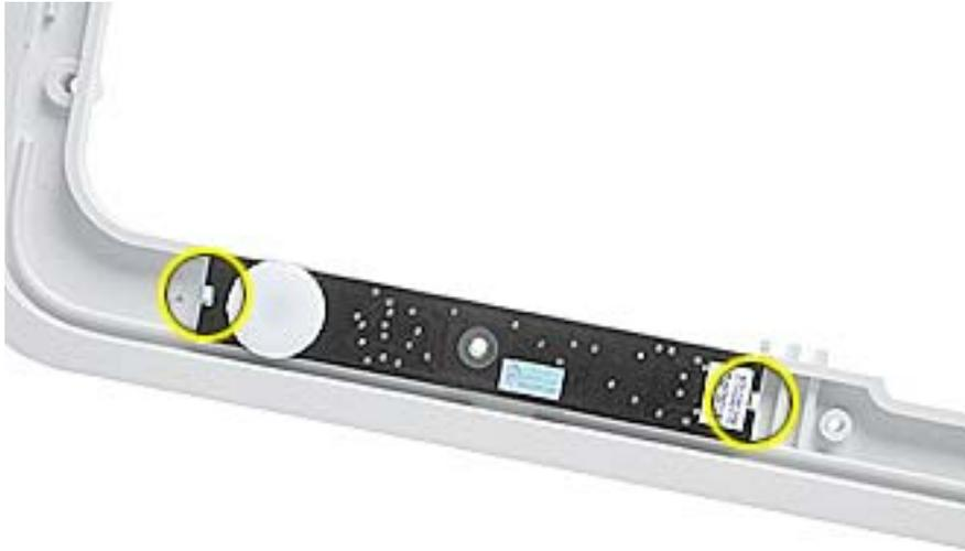
**Replacement Note:** When reattaching the cable connector, the board will be springy. Verify secure connection.
