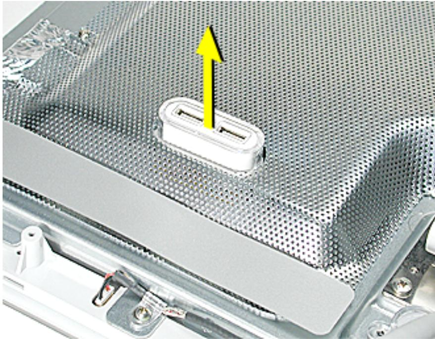
2. Remove ten Phillips screws on the EMI shield.
