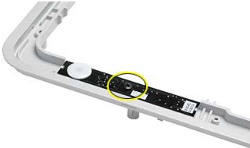
**Replacement Note:** Make sure that the rubber boot is in place on the inner bezel before installing the switch board.
