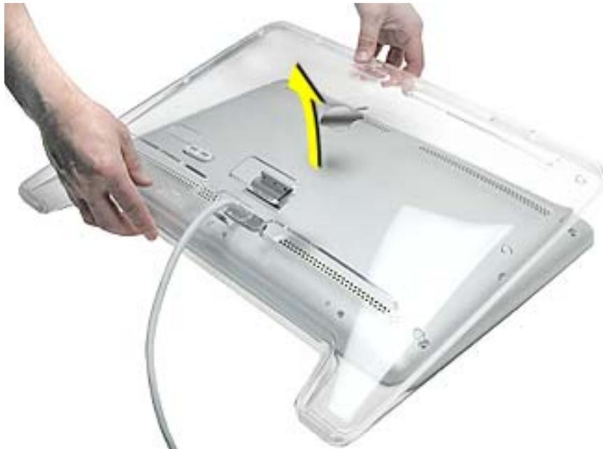
**Replacement Note:** Verify that the USB socket cover is in place, and that the arrowheads on the USB icon point up.
