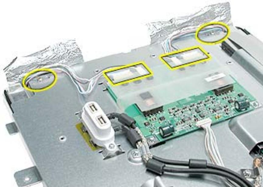
3. Disconnect cable connectors to the display panel.
